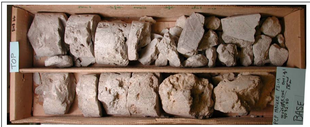
Figure 2A. Panuke PI-1A core #1 – dolomite F-M crystalline with vuggy and intercrystalline porosity. Only 1.1 m recovered from 4029.28 m to 4032.8 m in AB 4.
