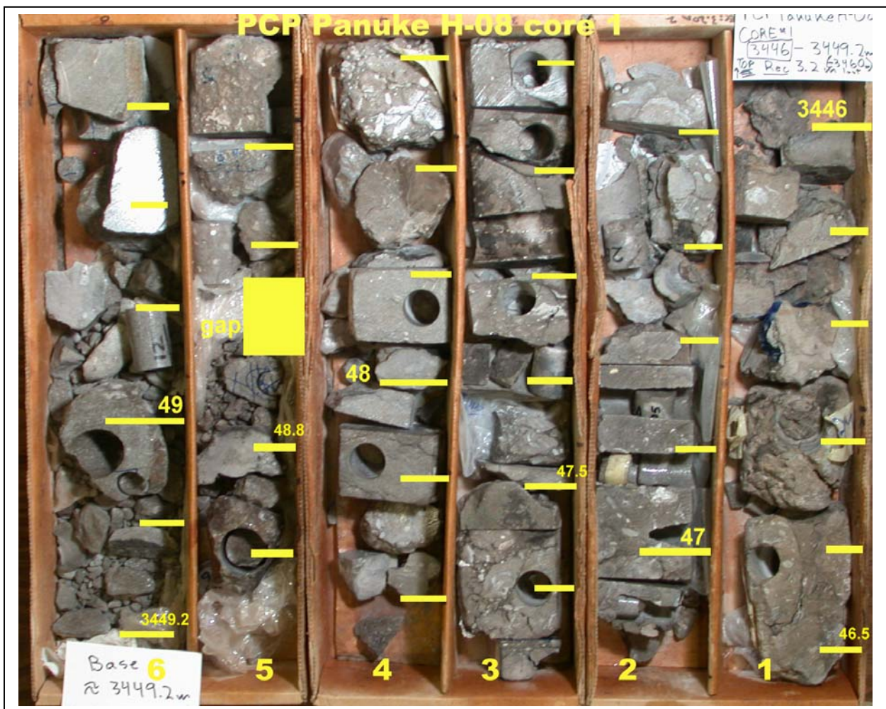
Figure 3A. Panuke H-08 core #1 – limestone of upper chaetetid-rich (coralline sponge) bioeroded rudstones to floatstones with minor colonial corals and common echinoderm grain- to packstones as matrix and dominant in lower core. Limestone has high amounts of micro-porosity and some brecciation. About 3.2 m recovered in AB 5.
