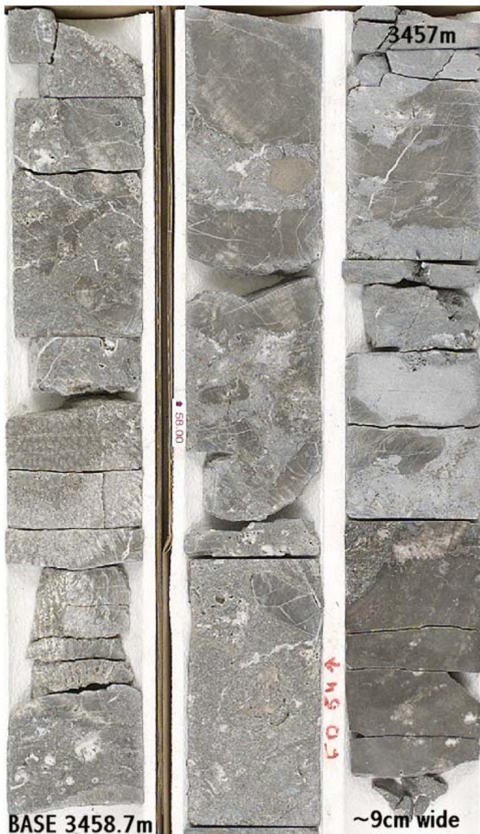
Figure 16: Core slabs, each slab 8.5 cm wide, dolomitic limestone, stromatoporoid-cabbage head coral rudstone in a skeletal packstone matrix, F-70 core 1, 3457 to 3458.7m (top left to bottom right). Note overturned coral head at base of core. Interpreted as shallowest water coral debris reef subject to storms or derived from such a reef and re-deposited on reef flat or proximal forereef slope.
